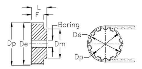
Belt width = - 16 mm = 138.2De Dm = 88 = 140.2Dp F = 21 L = 31 Pre-drilled = 10
